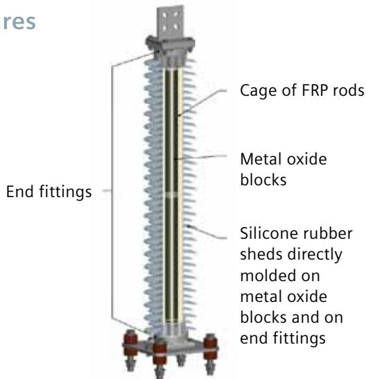
Siemens' Cage Design ensures high mechanical strength and safe overload performance. It is characterized by the use of silicone and fiberglass-reinforced plastic (FRP) rods as housing materials. Reliability is guaranteed by the direct molding of the silicone rubber onto the MO blocks and the FRP rods. This ensures the total embedding of all components free of bubbles and gaps, thus preventing any partial discharge or moisture ingress.
