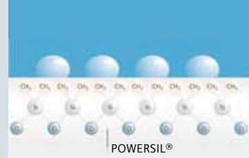
Hydrophobic effect on Siemens 3EL surge arrester due to alignment of methyl groups in silicone polymers.
