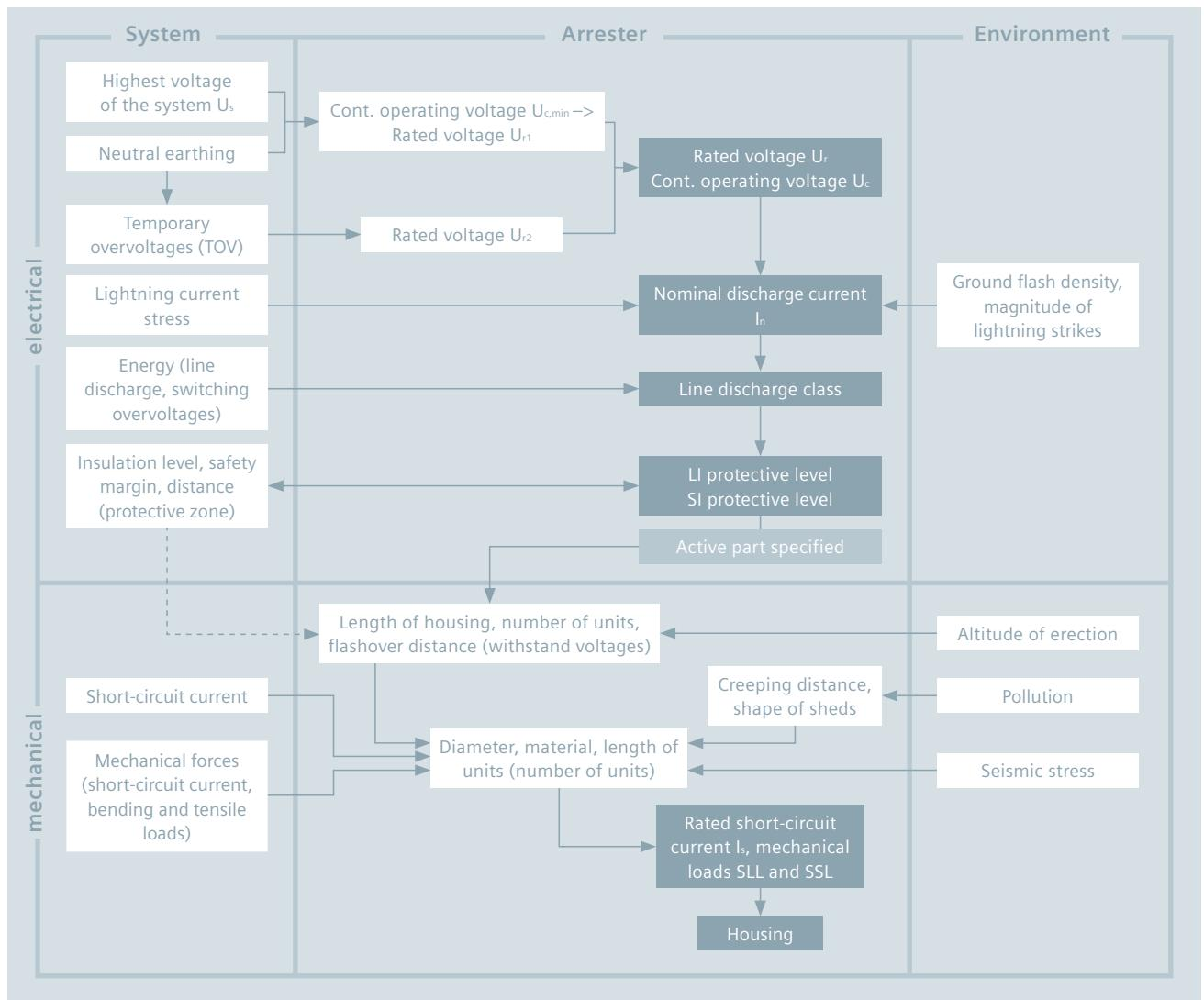
Fig. 1: Configuration procedure for an MO surge arrester
