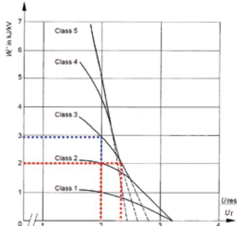
Specific energy in  $\text{kJ/kV}$  of rated voltage dependent on the ratio of switching impulse residual voltage  $U_{res}$  to the r.m.s. value of the rated voltage  $U_r$  of the arrester (from IEC 60099-4)
