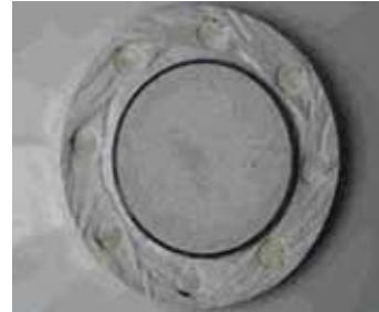
Horizontal cut of a cage design arrester
