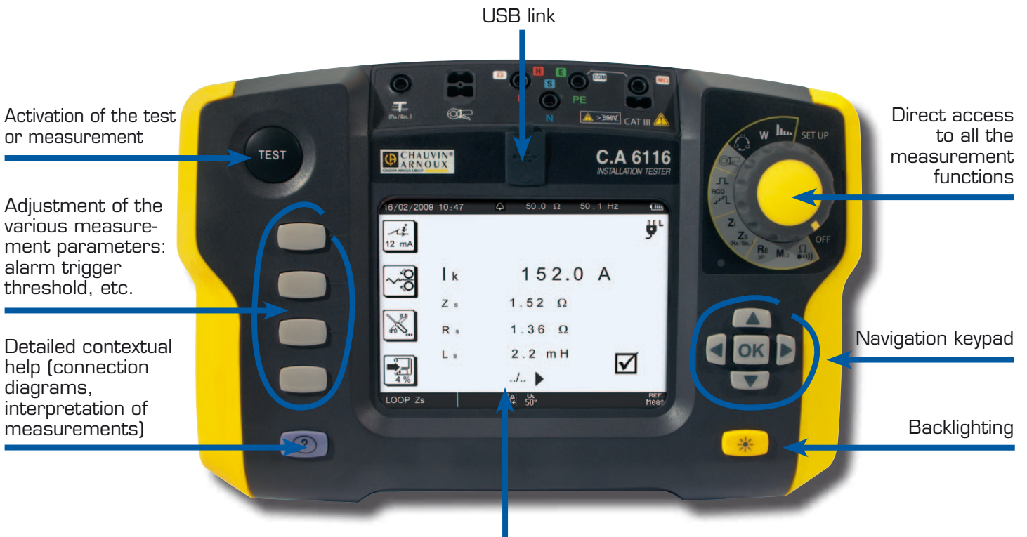
Wide graphic screen for excellent legibility and simple navigation within the instrument
